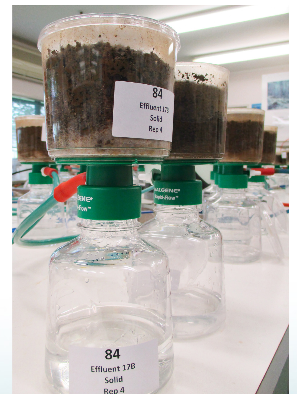
Example of a filtration unit used to incubate the effluent amended soil
