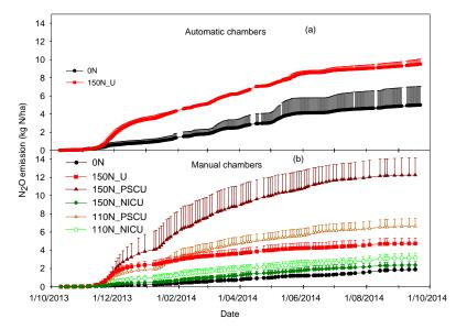
Figure 1. Cumulative N<sub>2</sub>O emissions (mean+SE) as measured with the automatic chamber (a) and the manual chamber (b) methods. 0N, 110N and 150N: fertilised at 0, 110 and 150 kg N/ha, respectively; U: conventional urea; PSCU: polymer and sulphur-coated urea; NICU: nitrification inhibitor-coated urea.
