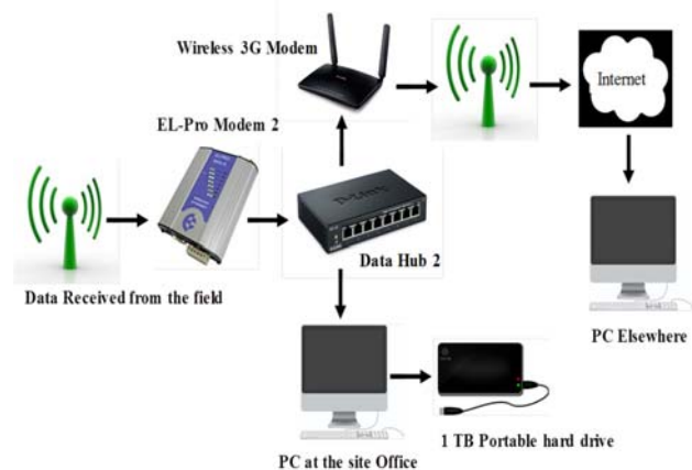
Figure 3. Schematic diagram of the equipment architecture in the field office.
