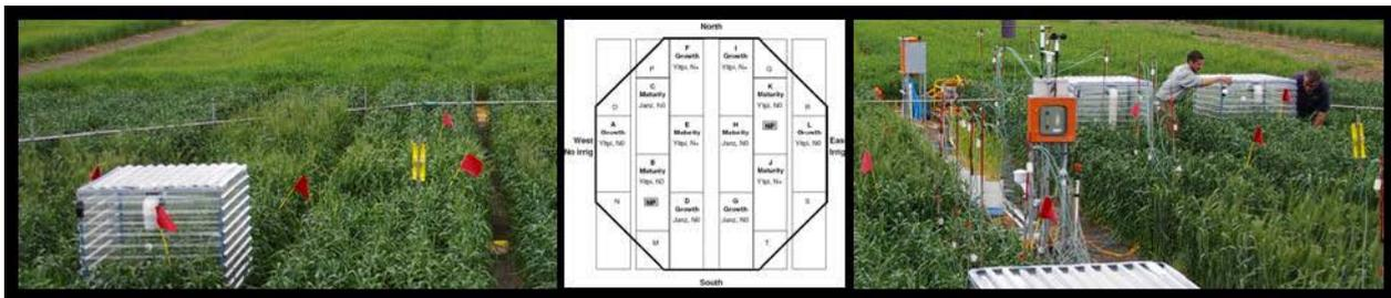
**Figure 1.** Design and layout of heat chambers within an AGFACE ring.
