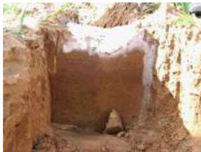
Figure 2: Paint infiltration test for visual assessment of infiltration (a) under wheel tracks and (b) under crop.
