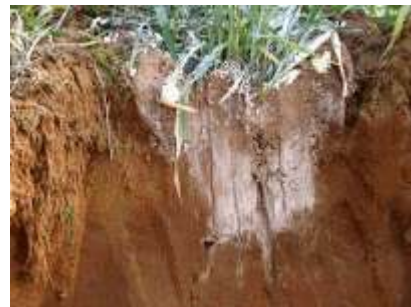
Figure 2: Paint infiltration test for visual assessment of infiltration (a) under wheel tracks and (b) under crop.
