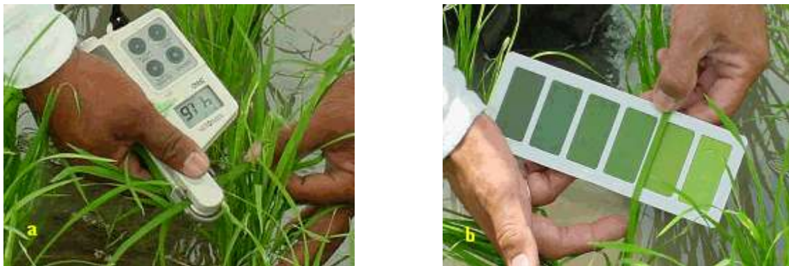
Figure 1. (a) Chlorophyll meter and (b) leaf color chart (LCC) for monitoring crop N status in situ in the field and applying N as per actual crop demand.
